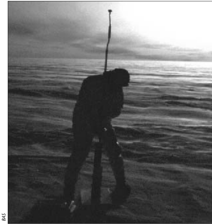
A glaciologist extracts surface ice core from the Antarctic ice sheet
